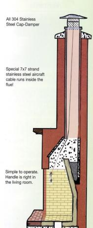
The main purpose of a damper is to seal the chimney when it is <u>not in use</u>. Heat rises, and if the chimney is not sealed when the fireplace is not in use, all the heat in the house goes up the chimney
