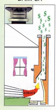
Huge heat loss occurs when a chimney damper doesn't seal properly or is missing or broken. You can't see it, the heat just goes out of the house. If your chimney's damper isn't sealing properly it's like leaving the front door open in the middle of winter!
